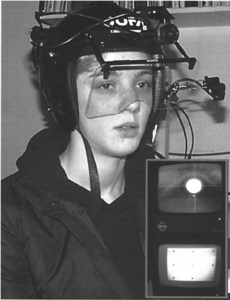
Figure 6.3 Eye-tracking technology allows psychologists to study visual search behaviour in expert athletes
