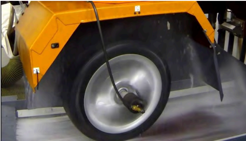
Hydroplaning is tested at the VTTI-affiliated Global Center for Automotive Performance Simulation (GCAPS).
