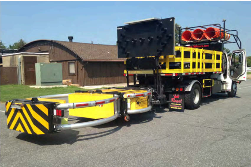
Despite being brightly colored, work vehicles like this truck-mounted attenuator can surprise drivers if they are not alert and prepared to respond to the unexpected.
